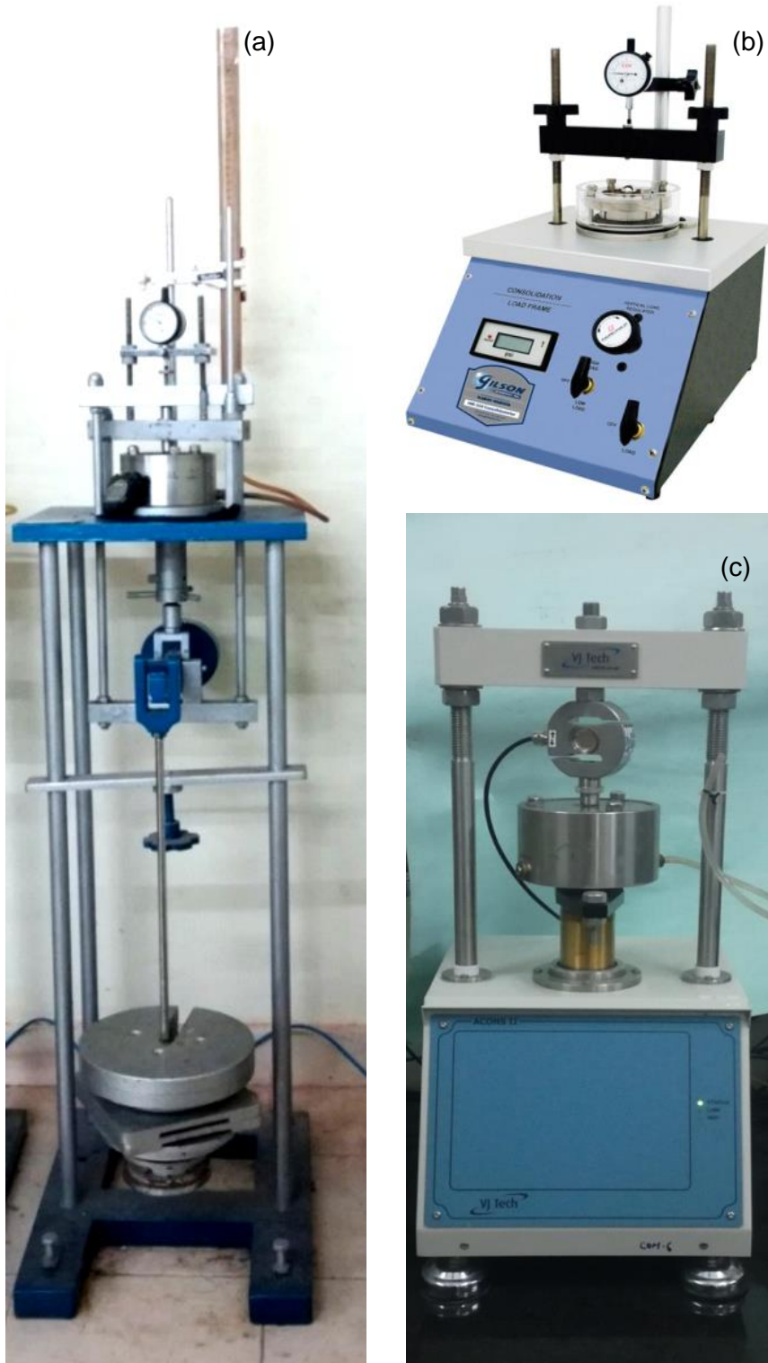
Figure 2.5: (a) Conventional loading Frame (b) Pneumatic consolidation frame ( www.globalgilson.com ) and (c) Automated consolidation frame
